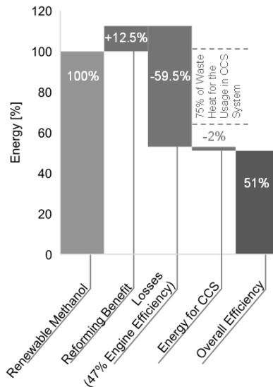
Fig. 4 Estimation of HyMethShip system efficiency
