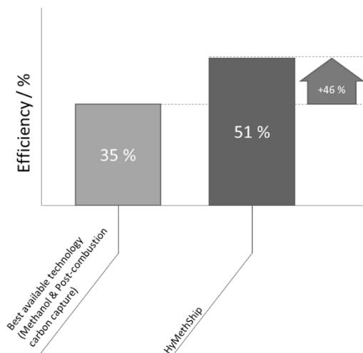
Fig. 2 Efficiency estimation for best available technology (methanol & post-combustion carbon capture) vs. HyMethShip (pre-combustion carbon capture)
