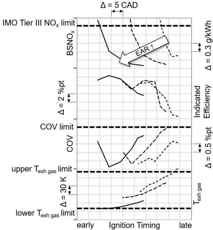
Fig. 6: EAR variation for hydrogen operation at nominal load
